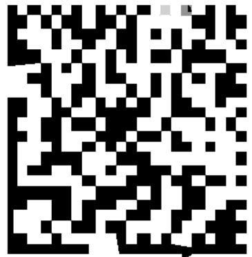
Fixed pattern damage
